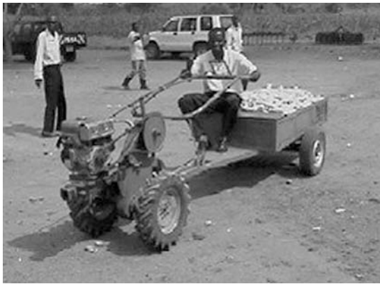
FIGURE 3.2. IRRI-Type two-wheeled tractor provides transport, can be used for tillage, harvesting, shelling, or threshing
